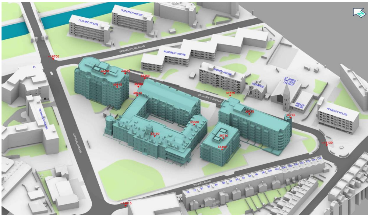
Figure 64 – CG Model of the proposed scheme used for the purposes of calculating daylight/sunlight impacts to neighbouring properties
